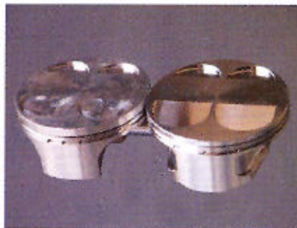
The new piston and the old one. The new version is bigger, but weighs less and is expected to last about three times as long.
